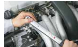
ONLY remove and fit glow plugs using a torque wrench.
