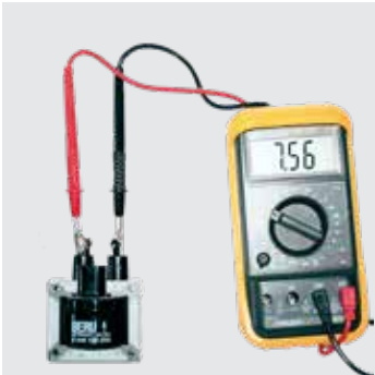
Secondary resistance test Test the secondary resistance: rated resistance for the secondary circuit at 20°C.
