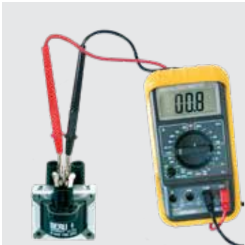
Primary resistance test Test of the primary resistance: rated resistance of the primary circuit at 20 °C.
