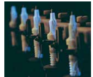
Testing insulators at 40,000 volts: BERU spark plugs have to demonstrate their reliability on the test rigs before being accepted for starting up in series production.
