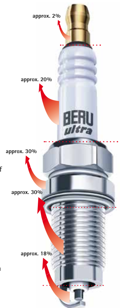
Heat conduction path of a spark plug
