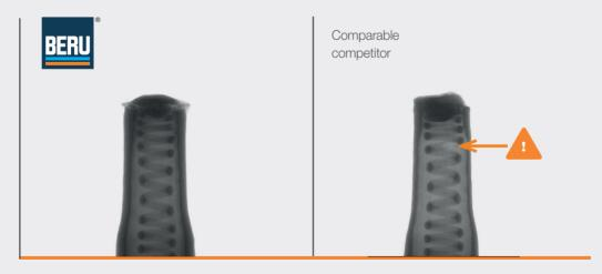
The thread spiral doesn't break, and passes the life cycle test with ease
